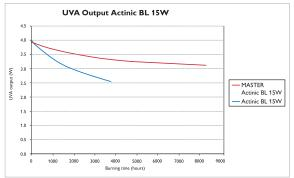
Thanks to the new environmental-friendly water based phosphor technology, the UVA output maintenance and lifetime have been significantly improved. As a result, the lamps provide maximum and reliable performance during the complete insect season, helping to safeguard a clean environment.
